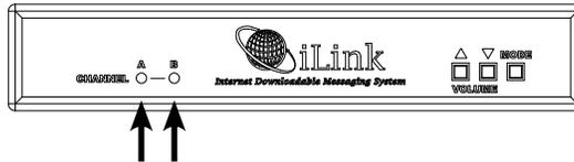
**Step 3:** After successful connection and download the LEDs (depending upon which CHANNELS are in use) will change to SOLID or FLASHING GREEN. This process can take anywhere from seconds to hours depending upon the size of download.
